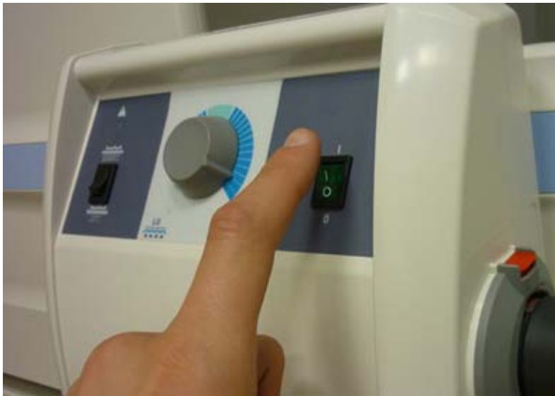
Fig. 8 Switching on SCU
